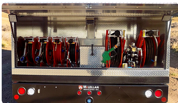
Fuel, oil & water hose reels.
