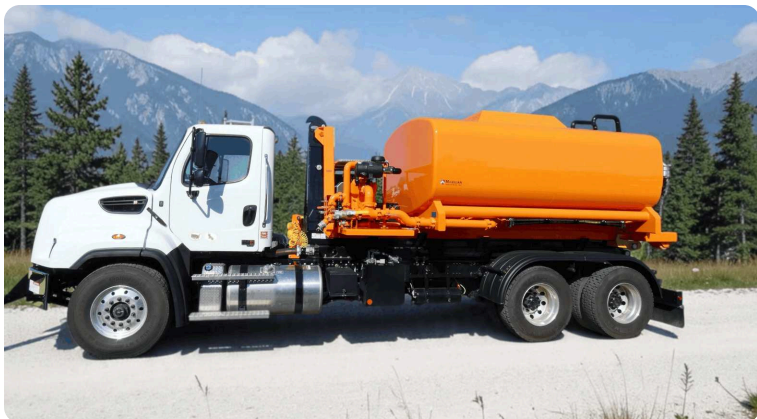
SELF-POWERED – 4x4 pump on its own Tier 4 diesel, so the skid works independent of the host truck
