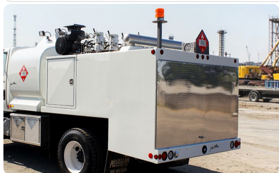
Compressor & pump bank, diamond-plate rear door.
