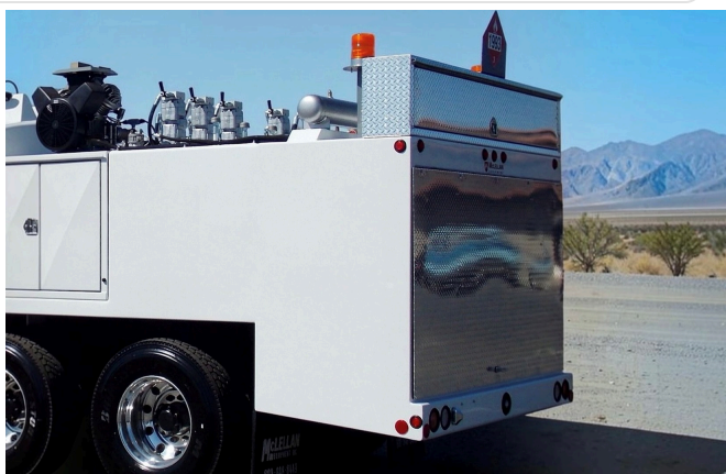
Pump and compressor deck, gauge/valve manifold, rear diamond-plated door.
