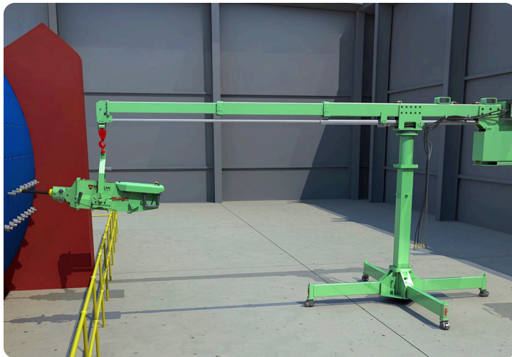
Jib crane suspending the Bolt Buster over the mill.
