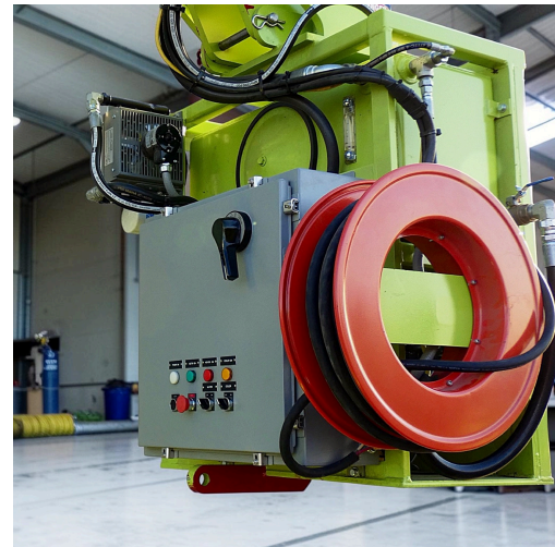
Control panel and hydraulic hose reel detail.
