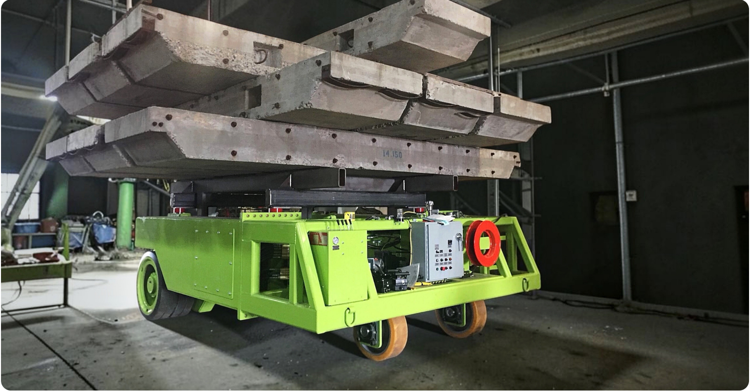
60 metric ton Feed Chute Transporter during acceptance testing.
