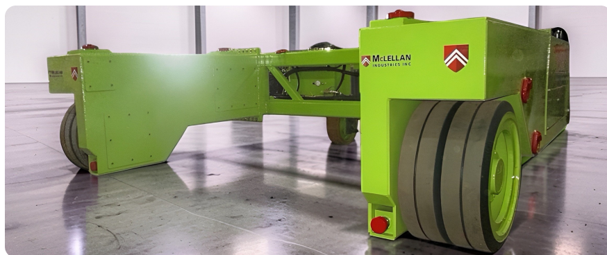
Heavy-duty drive wheels, U-frame chassis, lift cylinder.
