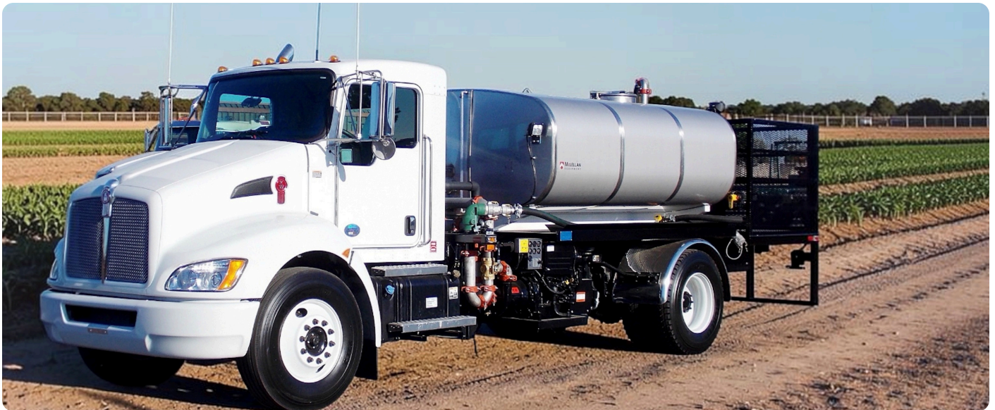
Pictured in base configuration — 2000-gallon stainless tank & integrated pump deck.
