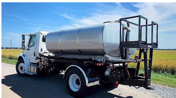
Rear crow's nest gates open - fill dome access.
