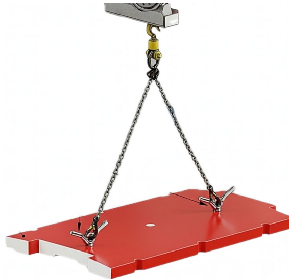
Chain sling lifting a mill liner plate.
