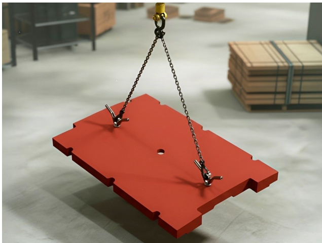
Chain sling and hook lifting a mill liner plate.
