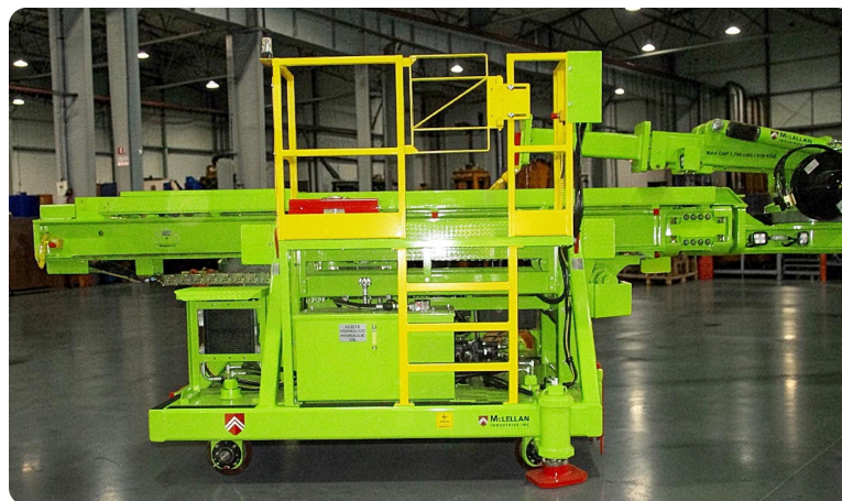
3-axis telescopic SAG mill liner handler, side profile
